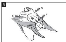
Assemble the radiator scoops with the screws (C).
