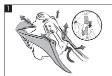
Remove the radiator scoops. Disconnect the fuel pump cover cable and the fuel connector as indicated in the diagram. Togliere i fianchetti. Sconnettere il cavo di
