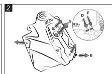
Remove seat screw and the screws on the side. Remove thetank screw (G), then empty any remaining fuel from the tank. Remove the (D)/(E)/(F) fasteners and remove the fuel pump.
