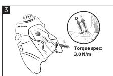
On the fuel tank Acerbis (A), reconnect the fuel pump (E) using the screws (H) with the original hardware (D)/(F).
