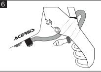
ATTENTION: fuel line addembly detail. Attach the KTM fuel line (F) to the Acerbis tank (A) as indicatedin the diagram. Make sure the fuel line isn't folded over, obstructing the fuel flow.
