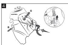
Place the Acerbis fuel tank (A) on the bike. Insert the tank screw(G). Insert the seat screws (B) as indicated in the diagram. Reconnect the fuel pump power cable and the fuel connector.
